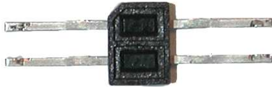
Fig. 6. The Sharp GP2L26 photointerrupter sensors are 3mm x 4mm, and they are located between the rails of the track at five points around the track layout. Each sensor can detect when a train passes over its track position.
